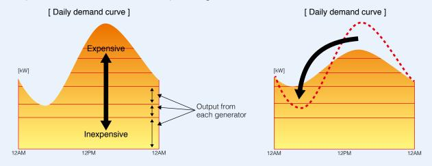
Chugoku Electric demonstrated that this technology could control the demand to be well aligned with the target curve.
