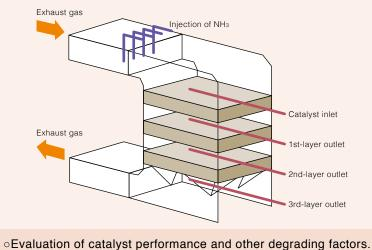
Design, supply, and regeneration of optimal catalysts
